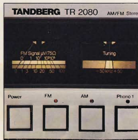
The large signal-strength meter gives easy to read indications up to 200 mV, and can be switched to read output power. An accurate center-tune meter ensures clearest reception of FM stereo broadcasts.
