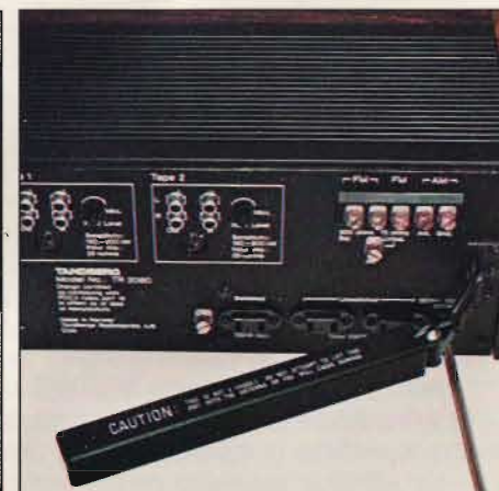
The built-in ferrite-rod AM antenna can be rotated through 270^\circ for optimum reception, and terminals are provided for external FM and AM antennae.
